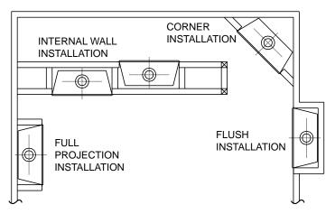
Figure 2 - Possible Locations for Installing Appliance
